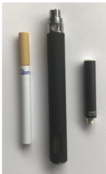
Figure 4. Study products. From left to right, cigarette substitute, ENDS battery, and ENDS cartomizer.
